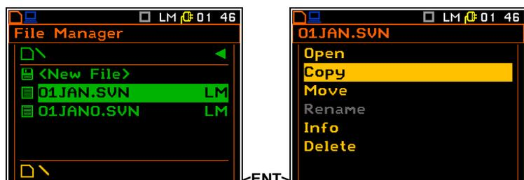
In order to perform this operation select the file/catalogue and press the **<ENTER>** push-button. After opening the list of operations select the **Copy** position and press the **<ENTER>** push-button again. The instrument then will propose to choose the target catalogue for copying. After selection of the target catalogue the user should press the **<ENTER>** push-button. The window with two options will appear: **Copy Here** and **Rename**.
