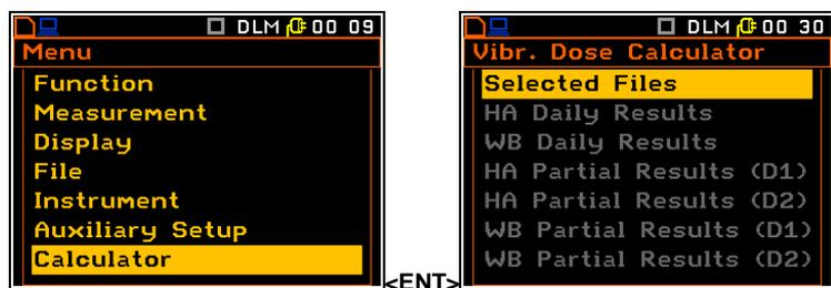
The **Selected Files** position is used to load data from the files with dosimeter results. It is possible to select up to 10 files for the calculations. The files are marked and loaded after pressing the **<ENTER>** push-button. The name of this file appears in a list as it is presented here.
