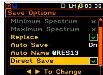
Press the **<ENTER>** and **<Alt>** push-buttons during the execution of a measurement causes, disregarding the option set in the **Direct Save** position, the message "Measurement in Progress" to be displayed.
