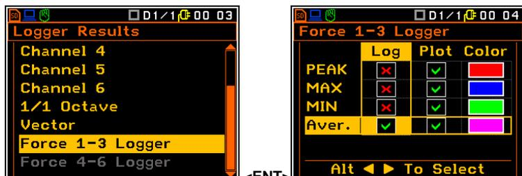
The force results in Newtons will be visible in Logger and Dosimeter presentation modes.
