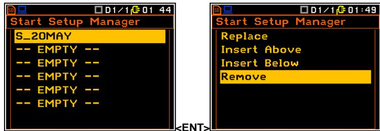
When instrument is restarted, it will show entries from the user-edited list of **Start Setup Manager** in between the **Whole-Body 1** and **Factory Settings** options. Selected setup will be loaded upon pressing the **<ENTER>** push-button.
