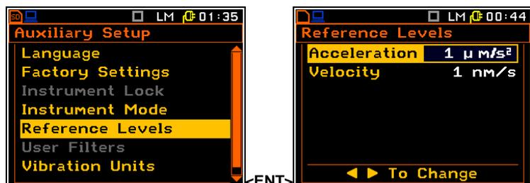
In the **Acceleration** position the user can set the reference level of the acceleration signal from **1 µms<sup>-2</sup>** to **100 µms<sup>-2</sup>**. In the **Velocity** position the user can set the reference level of the velocity signal. It is possible to set this level from **1 nms<sup>-1</sup>** to **100 nms<sup>-1</sup>**.
