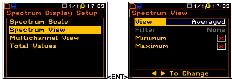
In the **View** position the user can select the different type of spectrum such as: **Averaged**, **Instantaneous**, **Max** or **Min**.
