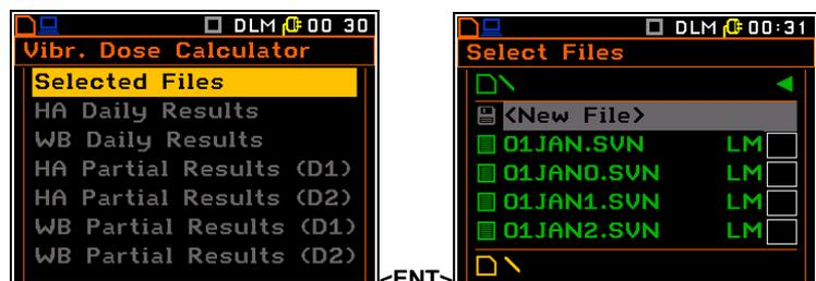
The **Invalid File Content** message is displayed when the selected file does not contain dosimeter data. The instrument waits for the reaction of the user by pressing any push-button except **<Shift>** and **<Alt>**. After that, it returns to the **Selected Files** list.
