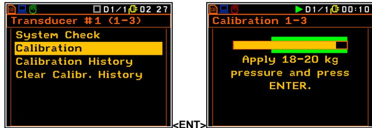
Please press the **<ENTER>** push-button when the scale indicates a value within the range that instrument asked for. Next please enter this value indicated by the scale in the Enter Force Readout box. Please press the **<ENTER>** push-button to proceed.
