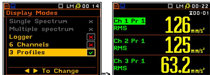
When all display modes in the **Display Modes** list are switched on they all are available and can be selected by means of the <Alt> and <^>, <v> push-buttons.
