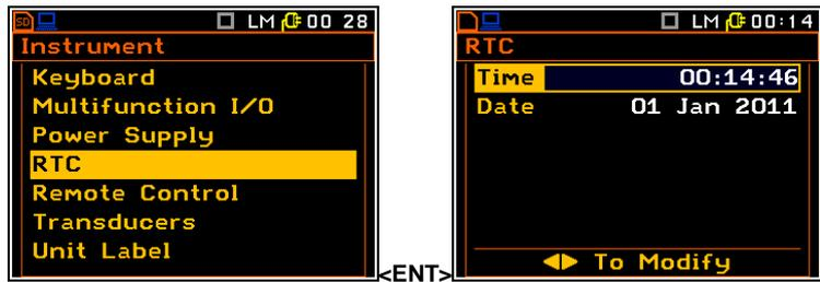
Editing the time is performed in the special window, which is opened after pressing the **<▶>** push-button. The selection of the correct parameter (hour, minute, second, and also day, month and year) is performed using the **<◀>**, **<▶>** push-buttons and the change of its value – using the **<▲>**, **<▼>** push-buttons pressed together with **<Alt>**.
