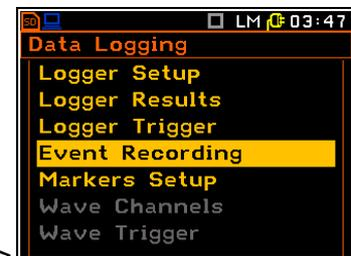
The **Event Recording** enables the user to activate recording of events and to set the parameters of event signal recording in the same logger file as for the regular time results history.
