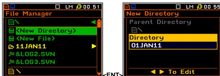
There is another way of saving results as a file in the internal or external memory than pressing the **<Save>** push-button. This can be done in the **File Manager** window by creating new file in the file system. To perform this function the user should enter the catalogue in which the new file will be created and press the **<ENTER>** push-button at the **<New File>** position.
