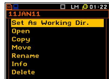
There are two options for storing result data in the internal or external memory. One option is to press **<Save>** push-button immediately after the measurement. Another option is to create **<New File>** in the **File Manager** window.
