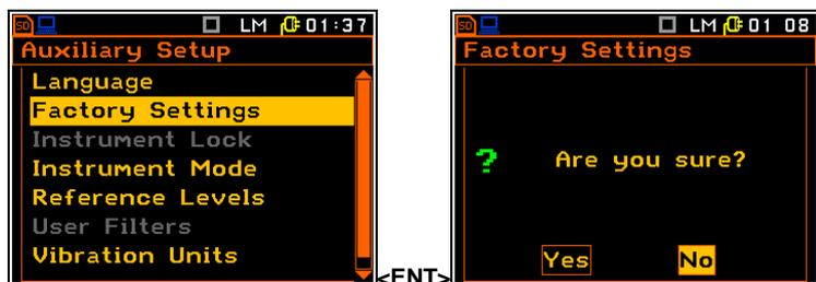
During the clearing process the message **WAIT...** is displayed. The following message is displayed after return to the default settings and the instrument waits for the user's reaction to press any key to continue.
