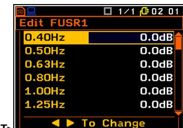
The opened window contains the centre frequencies of the filters and their coefficients:
