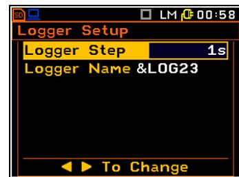
The **Logger Name** enables the user to name the logger file. The default name is **LOG#** for **Logger** files and **&REC#** for **Wave** files. The name can be up to eight characters long. After pressing the <Left>, <Right> push-buttons, the special window with text editor function is opened for editing.
