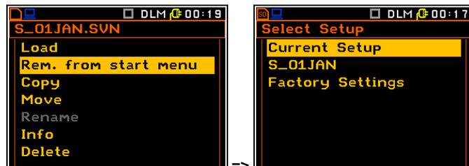
To get information about the setup file the user should select the file and press the **<ENTER>** push-button. After opening the list of operations select the **Info** position and press the **<ENTER>** push-button again.
