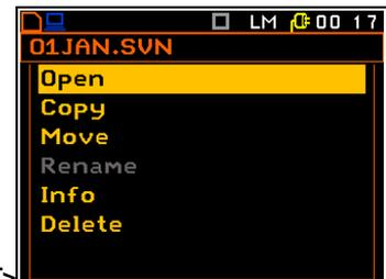
When the memory disk is selected after pressing the **<ENTER>** push-button the list of operations on disk appears.
