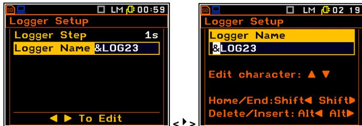
The edited name is accepted and saved after pressing <ENTER>. The special warning is displayed in case a file with the edited name already exists in the memory. The instrument waits then for a reaction of the user (any push-button should be pressed except <Shift> or <Alt>).
