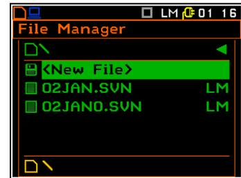
The list of operations on files saved in the **Internal** memory differs from **SD Card** by one position. It is not possible to rename the files saved in the **Internal** memory and thus the **Rename** position in this list is not active.
