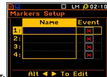
window that is opened by means of the <◀>, <▶> push-buttons pressed together with <Shift> or <Alt> while the cursor is on the **Name** position.
