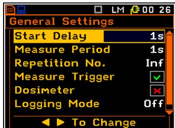
If the parameter has a numerical value the user may keep pressing the **<◀>** or **<▶>** push-buttons (or pressed together with **<Shift>**) longer than 1 second to speed up the selection. In this case the parameter
