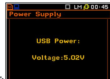
The instrument can be powered from four AA rechargeable or standard alkaline batteries or from the USB interface when its USB Device socket is connected by means of the cable to a PC or USB power supply such as the SA 54. The view presented on the display for each powering sources is different. The current battery voltage is displayed together with its approximate state (in the graphical form).
