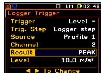
The **Level** position enables the user to select the value of threshold for
