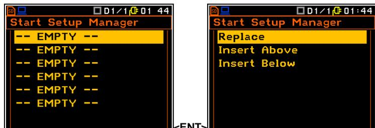
Please select setup file from the instrument memory and press the **<ENTER>** push-button to assign it to the desired position in the **Select Setup** menu.
