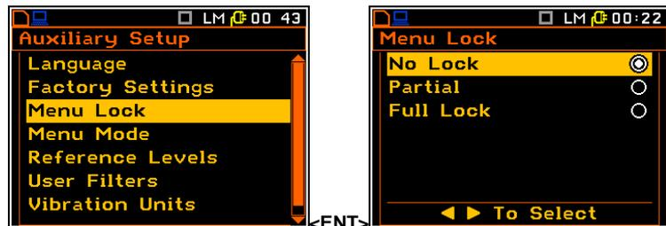
The activation of **Partial** results in locking access to the **Menu** options, which are responsible for measurement parameters. In the case of **Full Lock** no one position from the **Menu** lists is accessible and after attempt of enter **Menu** the **Menu Lock** window appears on the display. The **Menu** is available after unlocking it.
