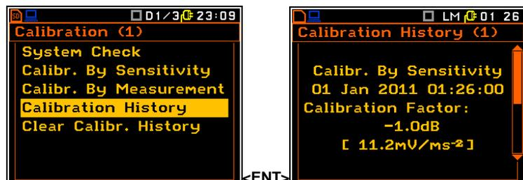
In order to review the calibration record, the user has to use the **<▲>**, **<▼>** push-buttons. The opened window will contain the date and time of the performed calibration measurement, the way the calibration was done (**Calibr. By Measurement** or **Calibr. By Sensitivity**) and the calibration factor (**Calibration Factor**) that was obtained.
