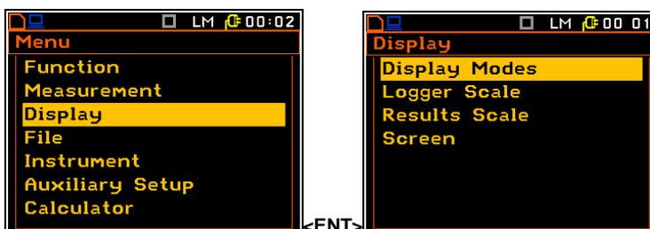
The **Display** list is used for setting the various parameters, which are mainly dedicated for the control of the screen display views. The list consists of:
