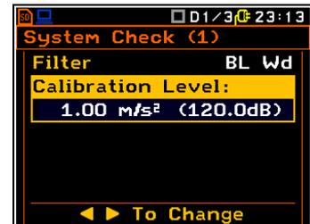
The measurement starts after 5 seconds delay. The system check measurement time is also predefined to 5 seconds. During the calibration period the **<ESC>** and **<Pause>** push-buttons do not operate but it is possible to stop the measurement using the **<Start/Stop>** push-button. Waiting for the calibration measurement to begin, a **Delay** is counted down.
