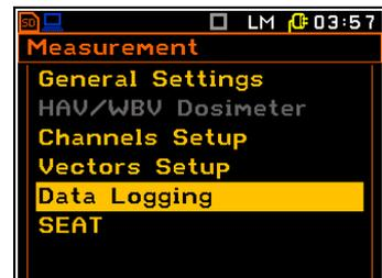
Depending on the selection of **Logging Mode (Logger or Wave)**, set up in the **General Settings** list, the **Data Logging** window will have a different view.
