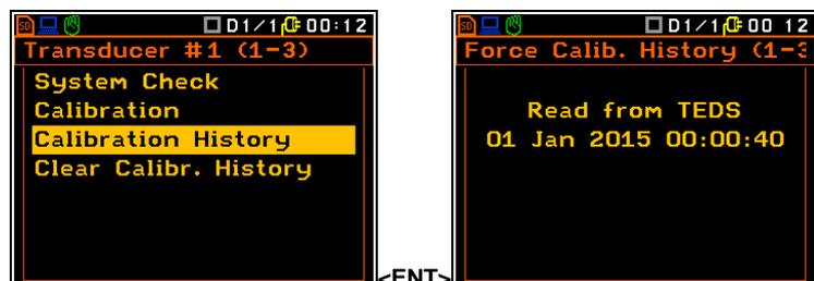
The user can clear all stored calibrations records of contact force sensor. In order to do this the user has to choose the position **Clear Calibr. History** and press **<ENTER>** to perform this operation.
